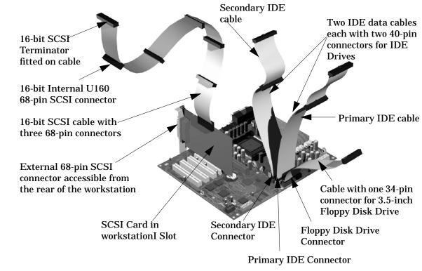
The total length of the external SCSI cables should not exceed 3 meters (approximately 10 feet).
